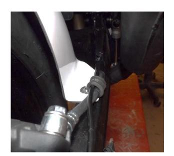
First remove the left hand side passenger foot rest to allow better access (2 x socket bolts).
