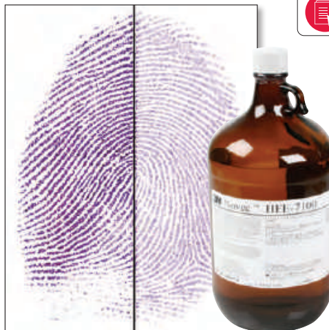
Comparison of latent print developed using Ninhydrin in 3M Novec Engineered Fluid HFE-7100 (left) and Petroleum Ether (right). ©1999 Jon T. Stimac, Oregon State Police (used with permission)
