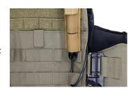
Route the antenna connector of the cable through the nylon loop at the bottom of the MAST harness from back to front.
