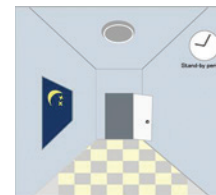
AT THE END OF THE WAITING TIME, NO MOTION IS DETECTED AND THE LIGHTS ARE TURNED OFF (OR KEPT ON AT THE WAITING BRIGHTNESS) IN THE THIRD STAGE.
