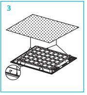
**3.** Clip the cable into the hooks of the backlit panel.
