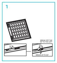
1. Remove the original ceiling tile for the backlit LED panel.
