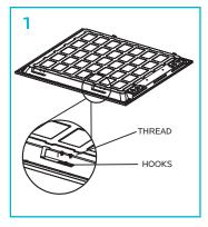
Turn off the electrical power, then make sure the backlit cable hooks are installed.
