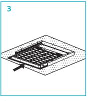
**3.** Slot the backlit panel into the bracket set.
