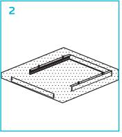
**2.** Fix 3 frames as bracket set on the ceiling as shown above.
