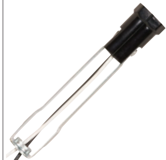
80-2487 6" Flange 26" #18 UL 1430 B/W Leads 105°C 1/8 IP - Inside Extrusion Double-Leg 80-2488 6" Flange 40" Leads 105°C 75W-125V
