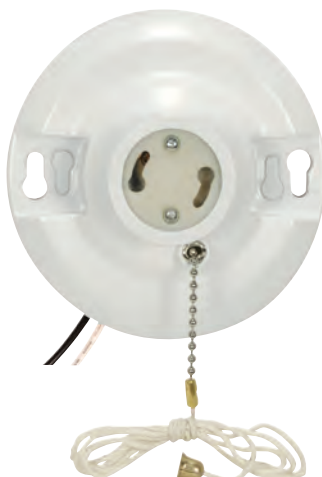
90-2470 White Phenolic GU24 On-Off Pull-Chain Ceiling Receptacle 6" AWM B/W Leads 105°C 4 1/2" Dia. 75W-250V
