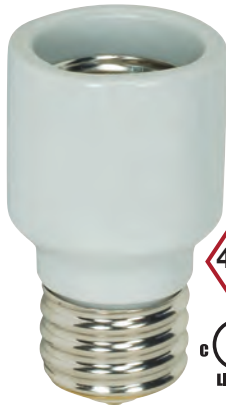
90-1801 Mogul to Mogul E39 - E39 Extender 4KV - Porcelain Overall Ext. 2 3/8" - 2 1/4" Dia. 1500W-600V
