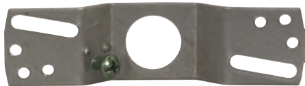
90-112 1" x 4" Screw Holes - 2 3/4", 3 3/8" and 3 1/2" Center to Center Center Hole Slips 3/8 IP with Ground Screw
