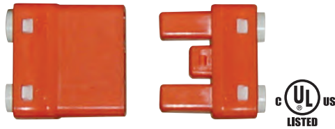
90-2536 Orange 2 Piece Snap Together Connector for Solid or Tinned Tip Wire: 18 AWG (Female Housing) 12/14 AWG (Male Housing) 3A-125V, 1.3A-277V 105°C
