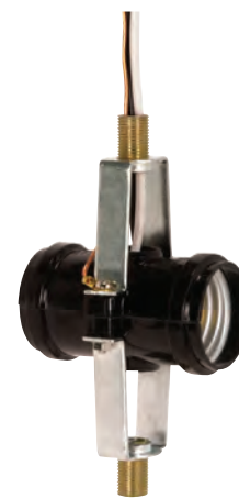
80-1380 1 3/4" 1/8 IP Threaded Top Bracket w/ 1/2" Nipple 1 3/4" 1/8 IP Threaded Bottom Bracket w/ 1/2" Nipple 12" AWM B/W Leads 105°C w/Ground Wire 660W-250V
