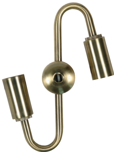
80-1709 Antique Brass Inside Wiring Only, 6" Centers 1/8 IP Top and Bottom
