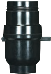
80-1106 Push-Thru 1/8 IP Cap w/Metal Bushing Less Set Screw 2 7/8" H x 1 1/4" Dia. 660W-250V
