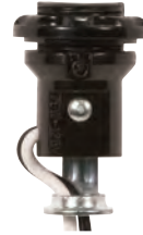
90-1557 1 3/4" w/Shoulder and Phenolic Ring 8" AWM B/W Leads 105°C Pulled Thru 1/8 IP Inside Extrusion 75W-125V
