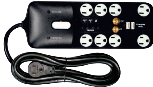
91-234 6' 14/3 SJT w/ Flat Plug 8 Outlet Surge Strip, Lighted On-Off Switch w/Circuit Breaker, 3000 Joules Rating, Surge Indicator Light, 2-2.1 USB Chargers, 2 Coax Cable Protection, 2 Adapter Receptacles, 15A-120V-1875W Packed 4
