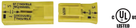
80-2010 Yellow (small) 2 Piece Snap Together Connector for Solid or Tinned Tip Wire: 18/12 AWG (Female Housing) 18 AWG (Male Housing) 6A-600V 105°C
