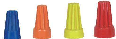
90-1852 Small Blue (105°C) 3 # 18 Max. 90-1419 Medium Orange (105°C) 5 # 18 Max. 90-1440 Large Yellow (105°C) 6 # 18 Max. 90-1421 Extra Large Red (105°C) 8 # 18 Max.
