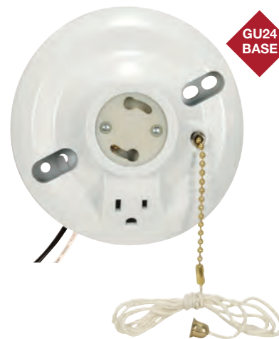
90-2484 White Phenolic GU24 On-Off Pull-Chain Ceiling Receptacle w/Grounded Outlet 6" AWM B/W Leads 105°C 4 1/2" Dia. 75W-125V
