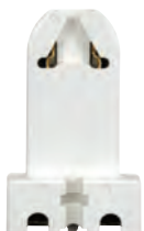
80-2025 Medium - T8 / T12 Lamps Screw Terminals - G13 Base w/Screw & Nut For Flush or Surface 2 1/2" H x 1 1/2" W x 3/4" Dia. 660W-600V
