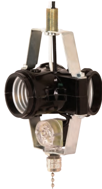
90-1587 3 Light Cluster Socket On-Off Nickel Pull Chain 1 3/4" 1/8 IP Threaded Top Bracket w/ 5/8" Nipple 1 3/4" 1/8 IP Threaded Bottom Bracket 8" AWM B/W Leads 105°C 660W-250V
