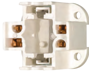
90-1550 18W 4-Pin Bottom Screw Down G24Q-2 & GX24Q-2 Base For: CF18DD/E & CF18DT/E Vertical Mount
