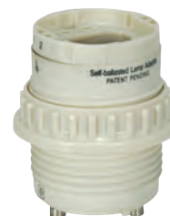
Phenolic w/Uno Ring 80-1851 120V, 60Hz, 0.30A 80-1857 277V, 60Hz, 0.30A 26W G24q-3 & GX24q-3 2" H x 1 1/2" W
