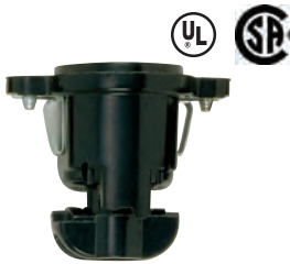
90-449 Snap-In Phenolic Sign Receptacle Lay-In Wiring - Twist Top For 14 & 18 GA Wire 1 7/8" H x 2 3/8" Dia. 660W-250V
