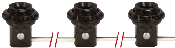
80-1912 1 1/4" with Shoulder and Phenolic Ring 9" Centers 18" Tail, AWM B/W Leads 150°C 75W-125V
