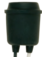
90-1097 Rubber Coated Pigtail Socket w/6" 14 GA 105°C Leads Aluminum Screw Shell 1 3/4" H x 1 3/4" Dia. 660W-600V
