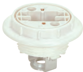
80-1506 13W 2-Pin Lampholder w/Uno Thread & Ring Height: 1 1/2" Push-In Terminals—Solid Wire w/U-Channel 1/8 IP Hickey, GX23 Twin, GX23-2 Quad 75W-600V
