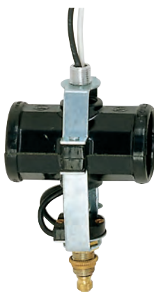
90-416 On-Off Brass Finish Turn Knob 1" 1/8 IP Threaded Top Bracket w/ 1/4" Nipple 1 3/4" 1/8 IP Threaded Bottom Bracket 6" AWM B/W Leads 105°C 660W-250V
