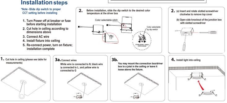
Our Slim Recessed Downlights can be used in drop ceilings if tile is capable of supporting the load. Use installation frame-in kits (RDL4-FRAME KIT or RDL6-FRAME KIT) to provide support as necessary.
