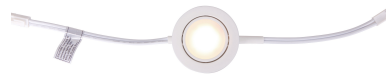
CPS1101-W-LED - 2.75" Puck 4 Watt LED; 250 Lumens, 3000k, 90 CRI, Dimmable 2.75"W x 1"H; Frosted Polycarbonate Lens Finishes: BZ, W
