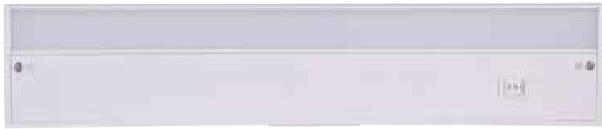
CUC1018-W-LED - 18" Light Bar 9 Watt LED; 600 Lumens, 3000k, 90 CRI, Dimmable 18"L x 3.63"W x 1"H; Frosted Polycarbonate Lens Finishes: BZ, W
