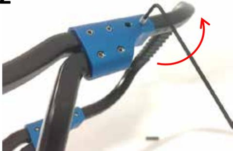
Use the 1.5mm Allen Key and remove Set Screws from front "U" section on 1 side only.
