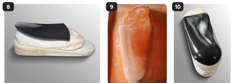
Carbon frame before vacuum forming
