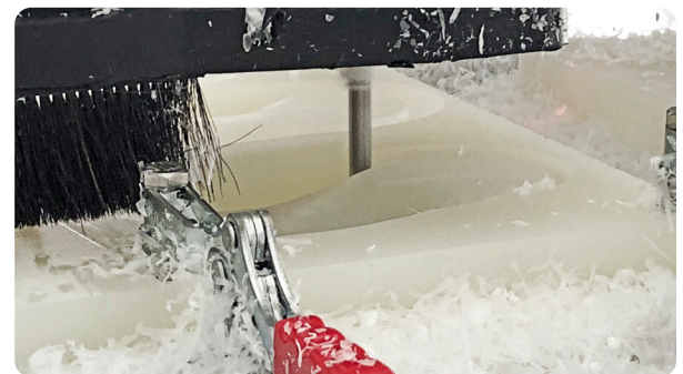
Mill Bit Cutting Polypropylene Frame
