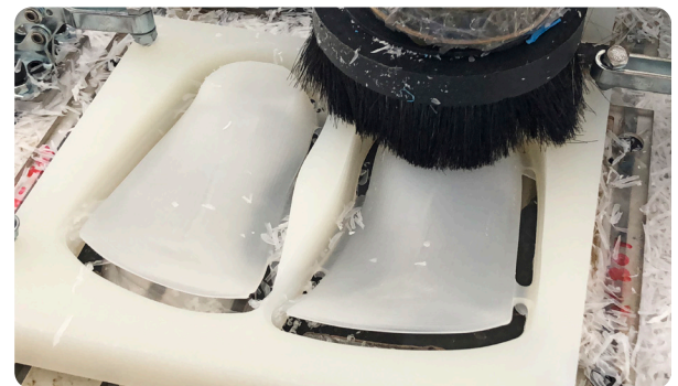
Polypropylene Frame Milling Process
