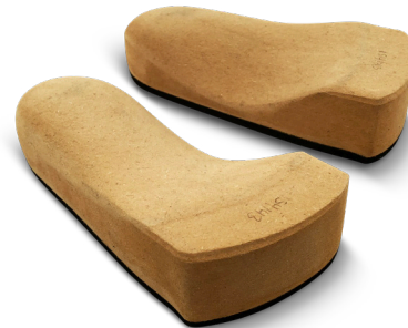
Milled out CAD CAM Positive Models
