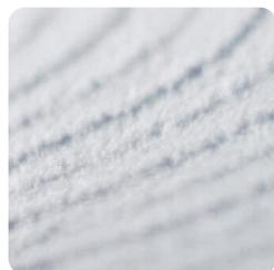
Close up of a SLS 3D printed orthotic. Layer thicknesses from Selective Laser Sintering (SLS) range from 0.060mm to 0.150mm. The lower the layer thickness, the higher the resolution and the longer it takes to make a 3D printed object of a given height.
