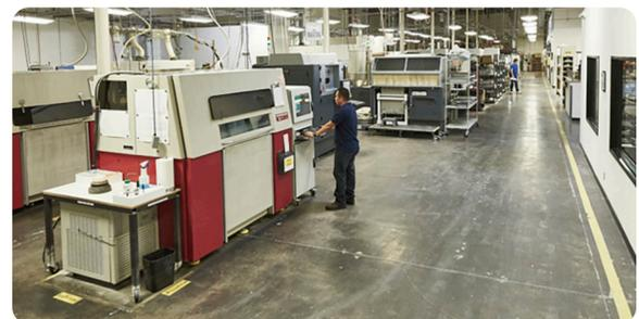
The 3D printers. 3D Printed SLS (selective laser sintering), is based on the melting of a plastic powder using a laser.
