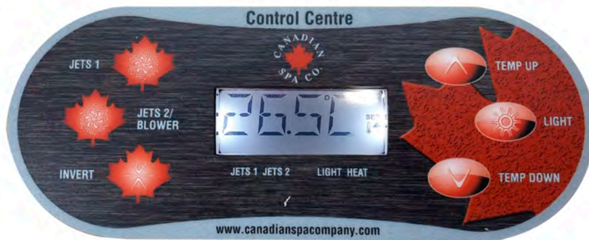
2 Pump Topside Control
