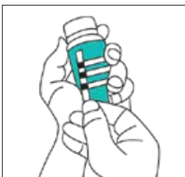
Balance water according to test strip readings
