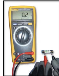
A FUSE WITH THE METER READING "GOOD"
