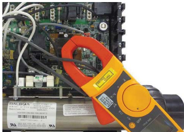
AMPERAGE HEATER TEST BP2100G1
