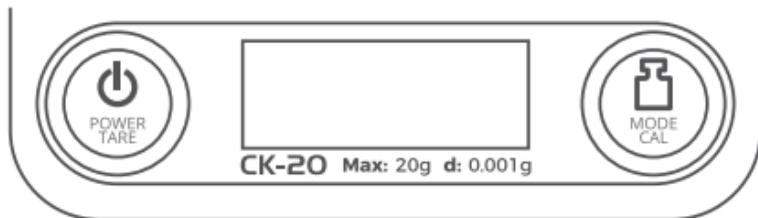
**Power/Tare:** Turns the scale ON or OFF. Zeroes the scale during normal weighing.
