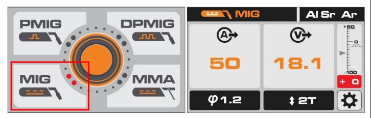
Normal MIG have no pulse, only adjust for wire feeding speed, pre and post gas time.
