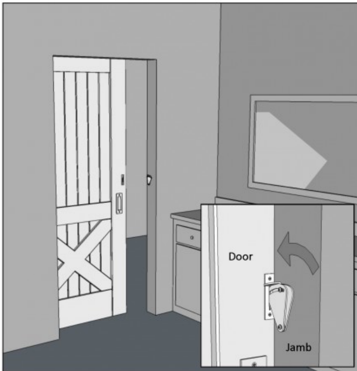
Teardrop mounted on Jamb
