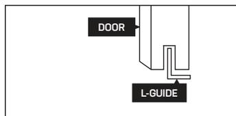
\*Doors must be in contact with door-guides at all sliding positions.
