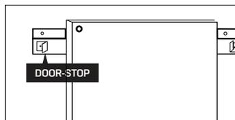
Install door-stops at the ends of the track to prevent doors from leaving the track.
