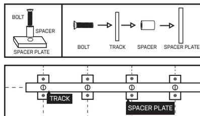
**\*NOTE: BE SURE TRACK IS MOUNTED SECURELY INTO SOLID BACKING**
