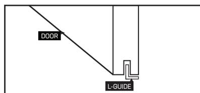
\*Doors must be in contact with door-guides at all sliding positions
