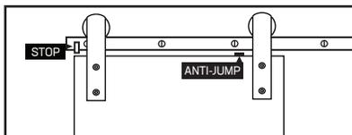
\*Door-stops are placed at the ends of the track to prevent doors from leaving the track.
