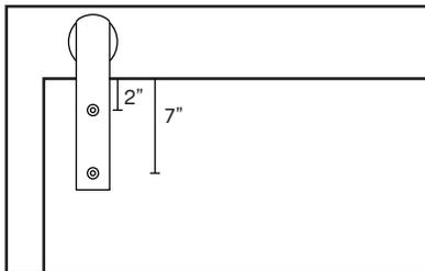
1. Place hangers on the top front part of the door (we recommend 2" in from the side of the door or center stile).
