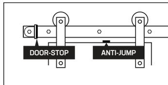
\*Door-stops are placed at the ends of the track to prevent doors from leaving the track.
