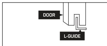
\*Doors must be in contact with door-guides at all sliding positions.
