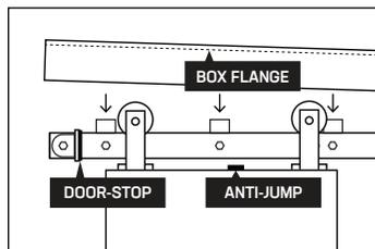
\*Door-stops are placed at the ends of the track to prevent doors from leaving the track.
