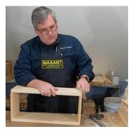
5. Wipe off any excess glue and dampen the end grain of each corner a bit so the joint dries snugly.
