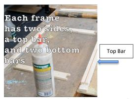
1. We recommend a good waterproof glue (Like Titebond III) on all parts before attaching with nails. Your frame will last for many years if it's built this way.
