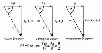
We see then that in its simplest form the power factor is the ratio of the equivalent series resistance to the impedance of the device.
