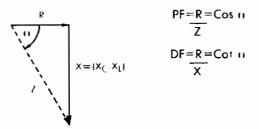
We can readily see that if X and Z are practically identical (which would be the case when approaches 90°), then the PF and DF would also be practically identical.
