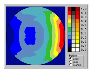
iCfg=2, nR=20, nPhi=20, spp=0.3 W/cm, Absorbed power = 0.1644 W/cm, Efficiency = 54.79 %, Wmax = 3.308 W/cm3
