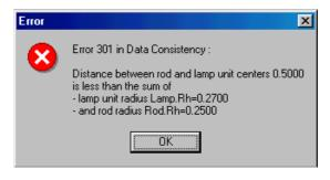
consistency check and in case of any data mismatch opens pop-up window with error diagnostics rather then starts the kernel file **OCCalc2.exe**. All input fields are subdivided into groups representing closely related parameters: General, Lamp/Diode, Laser Rod, and Configuration. Groups are placed in separate worksheets, each of which can be brought to front by clicking on **General**, **Diode**, **Laser Rod**, or **Config n** bookmark at the top row.
