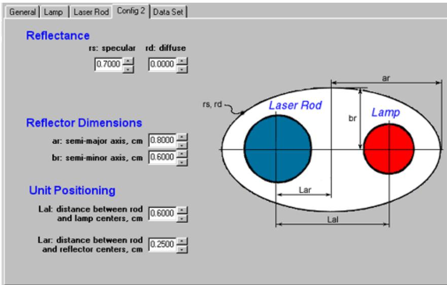
**Composition:** laser rod, lamp, and elliptic reflector.
