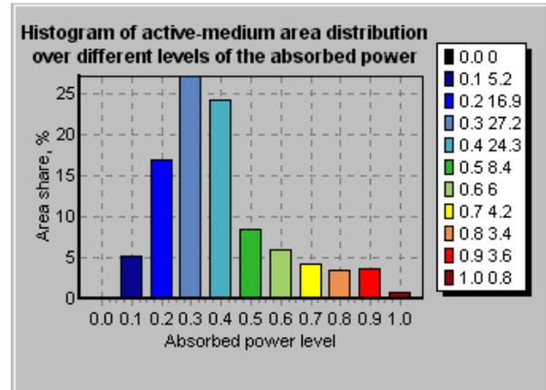
The button **1D** allows passing to another representation of the data obtained: a histogram. Being pressed, this button replaces the 2D plot by its one-dimensional counterpart in which the area share of each absorbed power level is plotted versus the value of the relative absorbed power density  $W_{rel}$ . Next click on the same button (now its caption is **2D**) brings us back to two-dimensional picture.
