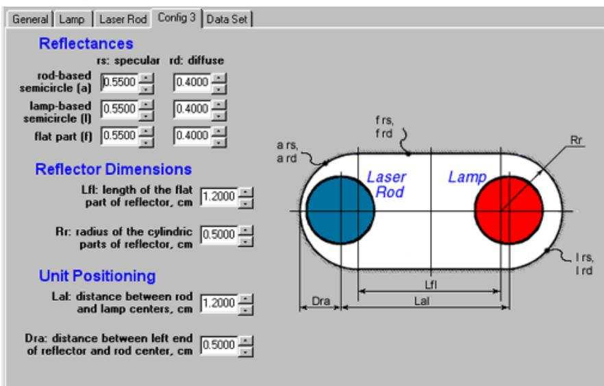
**Composition:** laser rod, lamp, and so-called compact reflector consisting of two flat surfaces confined at the ends by adjoining semi-cylinders.
