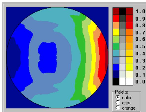
$iCfg=2$ ,  $nR=20$ ,  $nPhi=20$ ,  $spp=0.3$  W/cm, Absorbed power = 0.1644 W/cm, Efficiency = 54.79 %,  $W_{max} = 3.308$  W/cm<sup>3</sup>
