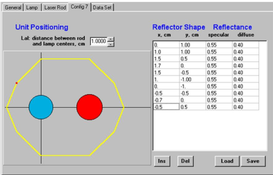
**Composition:** laser rod, lamp, and reflector described by a polygon.
