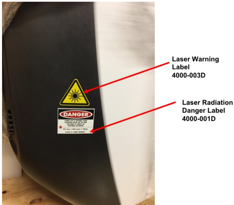
Figure 3-10. Labels, front of the POLYLASE MX Laser
