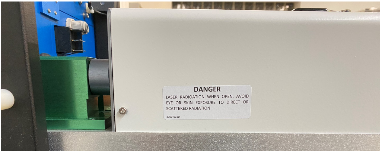
Figure 3-13. Laser Head Cover Label
