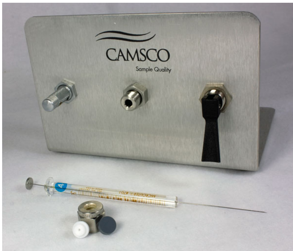
Figure 3A: Photo of the PTFE needle guide (white) and the septum (grey) inside the injection port
