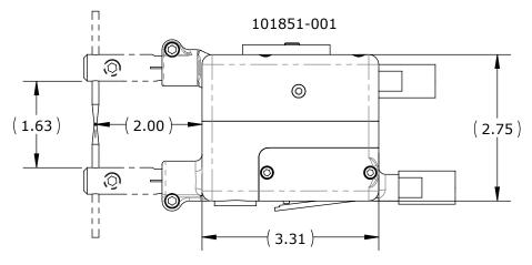
**MODEL DESCRIPTION:** 20 OZ. PNEUMATIC MINATURE SCISSOR GUN WITH AIR COOLED CABLES AND ADJUSTABLE STROKE. ELECTRODE FORCE = 15 LBS. AT 80 P.S.I.
