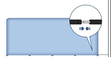
Make sure that the power cords have been pulled through the holes in the back of the fabric before zipping.
