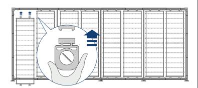
Connect the poles, then rotate the feet connected to the bottom poles perpendicular to the frame.
