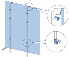
Adjust the tube's height and tighten in place with the twist knob.
