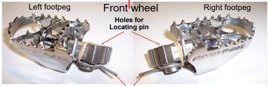
Spring legs lean against the motorcycle frame and are compressed when pegs are moved into position and locating pins are inserted. Trim to length if required.
