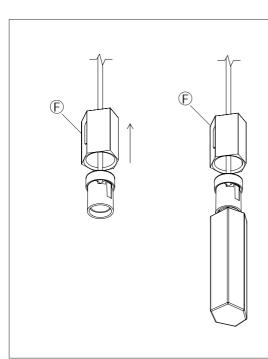
Lift the metal pendant sleeve (F) and screw the bulb firmly into the socket. Take care to prevent the metal sleeve from dropping onto the glass bulb.
