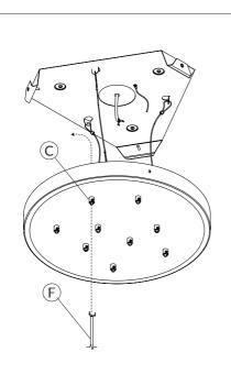
Thread all nine pendant cables  $\bigcirc$  though ceiling plate cord grips  $\bigcirc$
