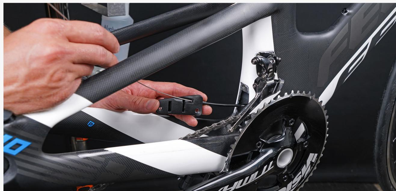
**Step 4:** Route the new inner wire. Note that the BatPac has a cable stop built in. Make sure that the housing (with housing end) is located in that cable stop before reinstalling the BatPac.
