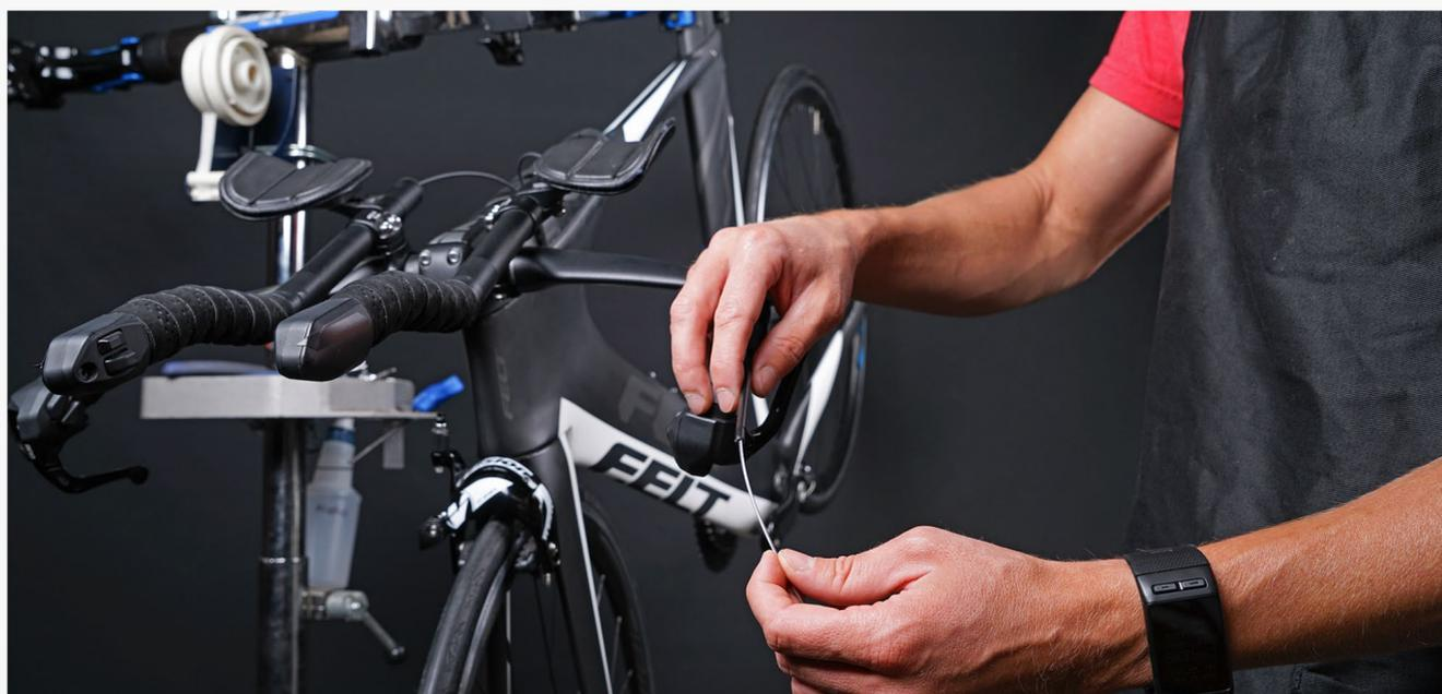
**Step B:** Using the existing housing, insert a spare brake wire starting at the brake lever side.
