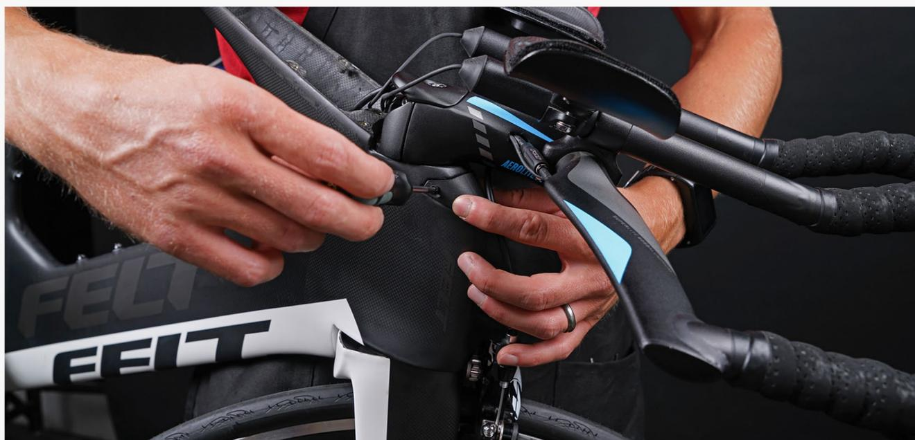
**Step 9:** Insert into the frame and attach with (2) M3 screws.
