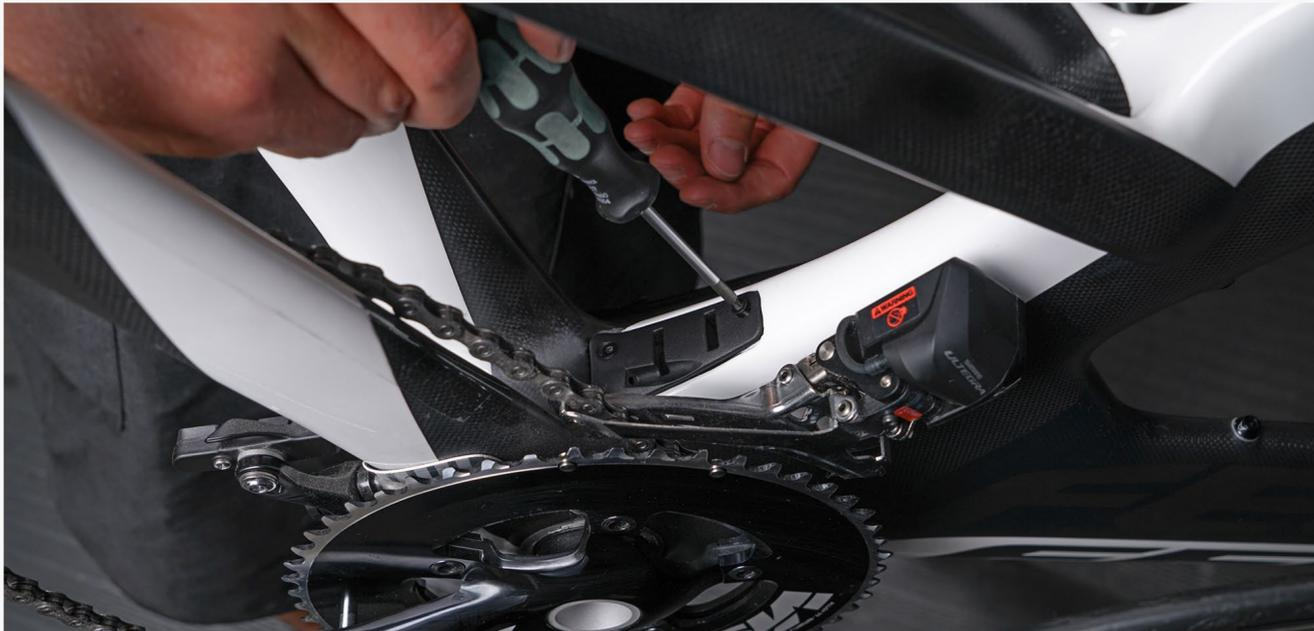
**Step 7:** Tighten the (2) M3 flathead screws to attach BatPac to the frame. Tighten to 2Nm.
