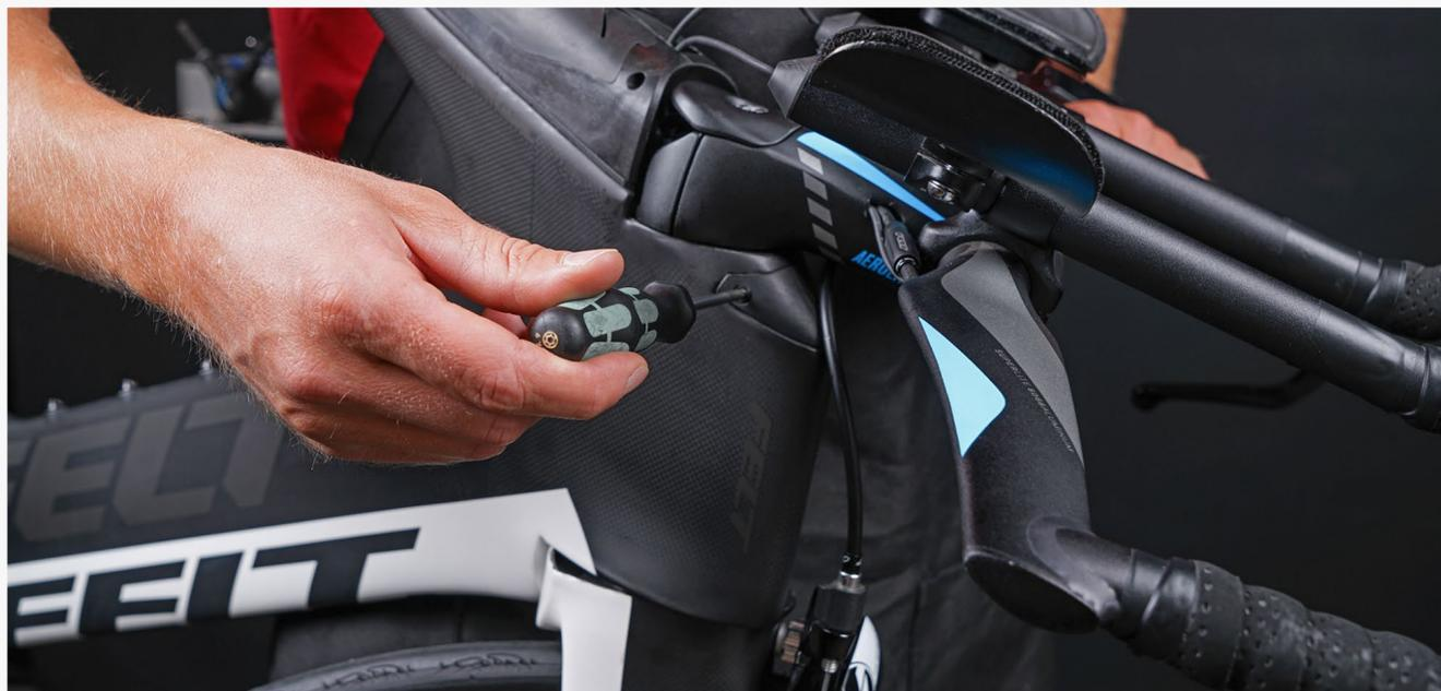
**Step 1:** Using a T9 Torx drive, unscrew the (2) M3 screws that attach the Di2 nose cone to the frame.
