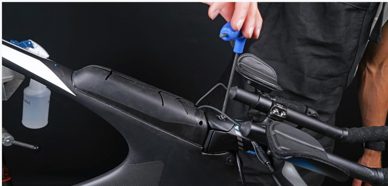
**Step 1:** Remove the stem top cap by unscrewing the Flathead M6 bolt with a 4mm hex wrench.
