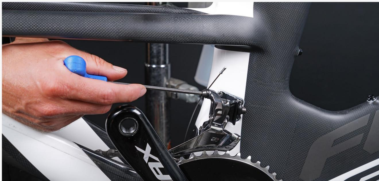
**Step 1:** Loosen the front derailleur screw and remove the cable end.
