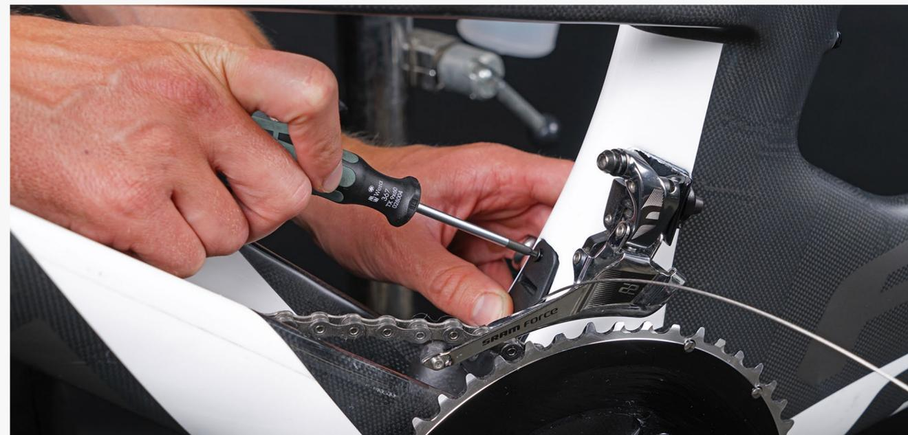
**Step 6:** Tighten the (2) M3 screws to attach the BatPac to the frame.
