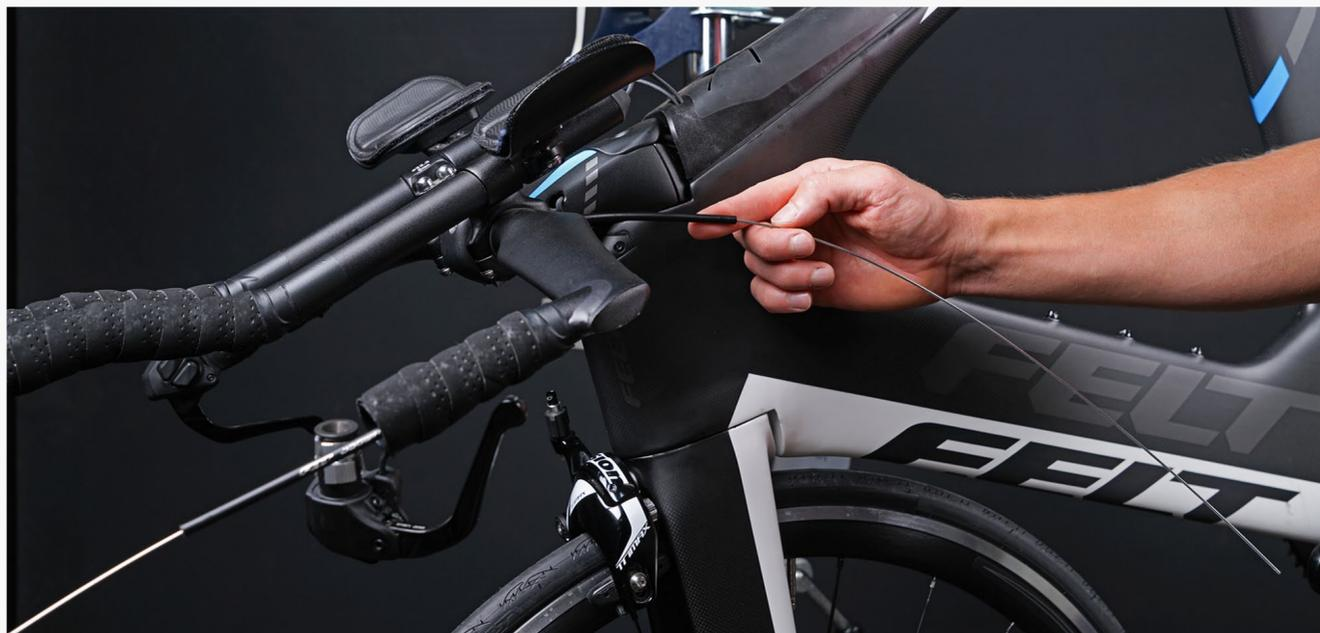
**Step D:** Insert new housing over the inner wire.
