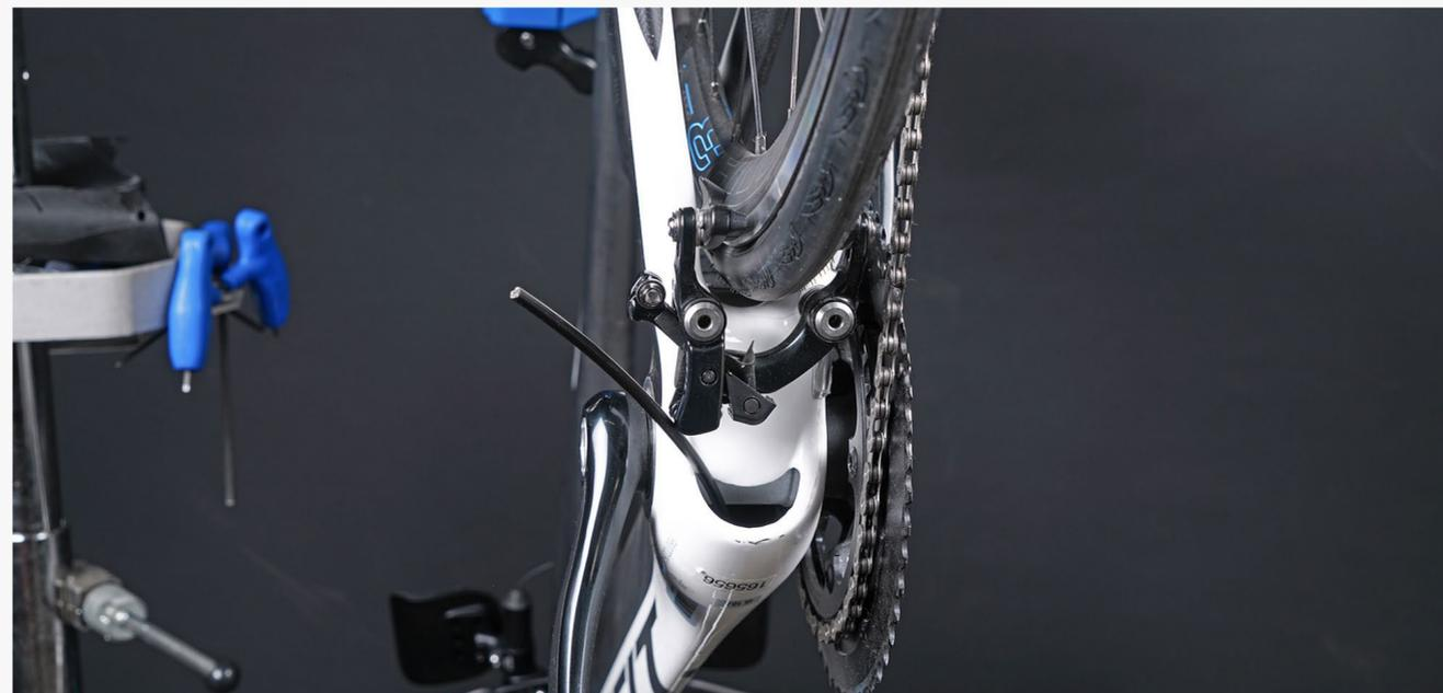
**Step 6:** If you are replacing the brake housing, remove the old housing and discard. Insert the new housing from the bottom up.
