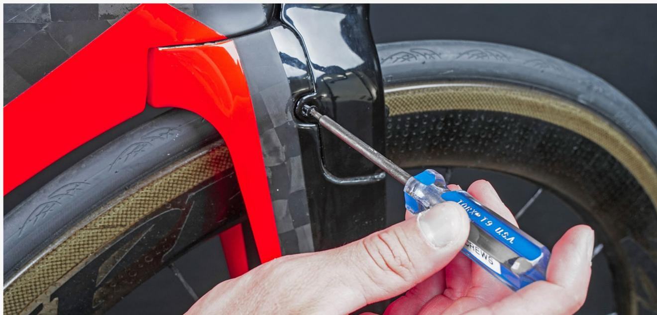
**Step 1:** Loosen the (4) screws that attach the brake covers. Use either a T9 Torx wrench or a 2.0 Hex wrench depending on the type of screws that your bicycle has.
