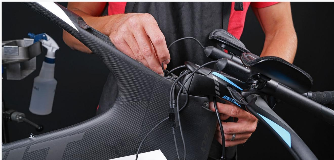
**Step 7:** To re-install Di2 wires, start at the frame opening and guide the cables around the steerer tube right below the top surface of the headtube. If you are not using Junction B to extend your shifter wires, then guide the shifter wires on the left side on the steerer tube. Otherwise, either side is acceptable. Do the same for brake wires and the single wire going down to the B junction by the bottom bracket.
