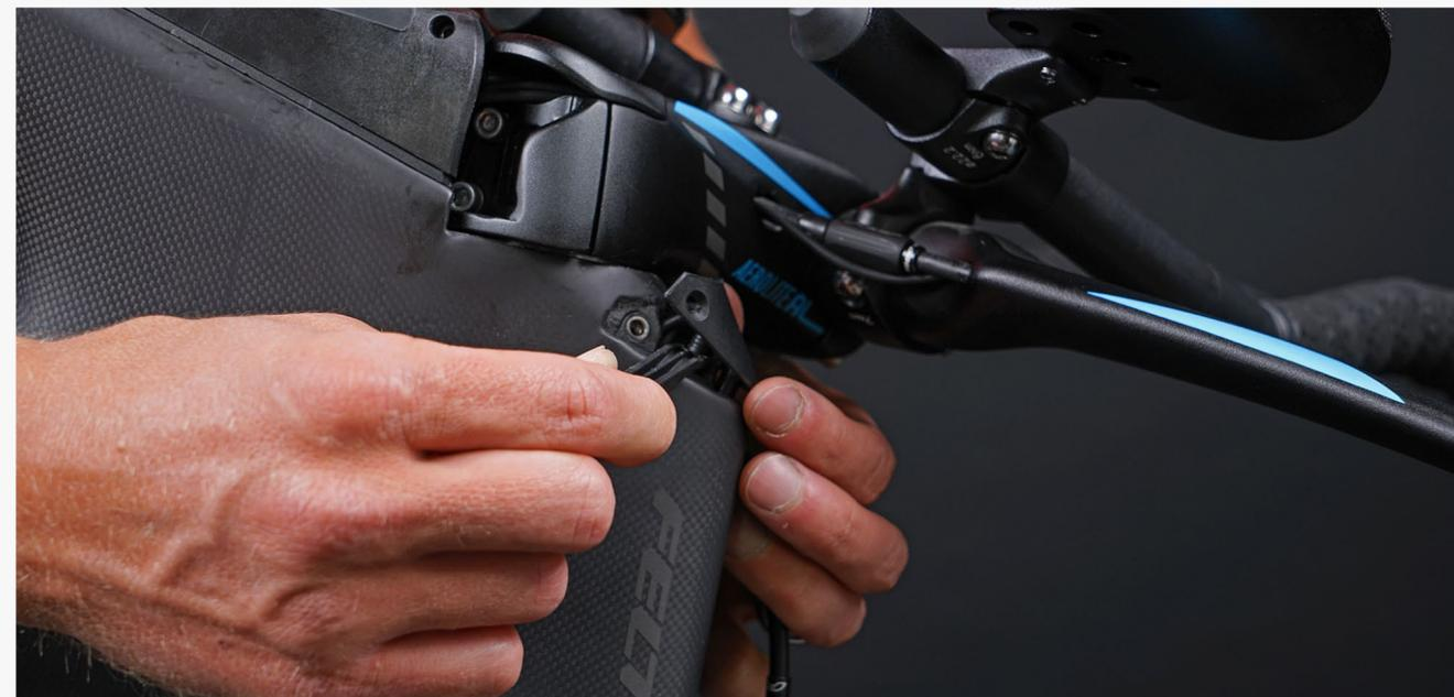
**Step 2:** If your Di2 wire length is limited, then you can first detach the Di2 wires from the A junction by using the Shimano Di2 installation tool while lifting the nose cone slightly out of the frame.
