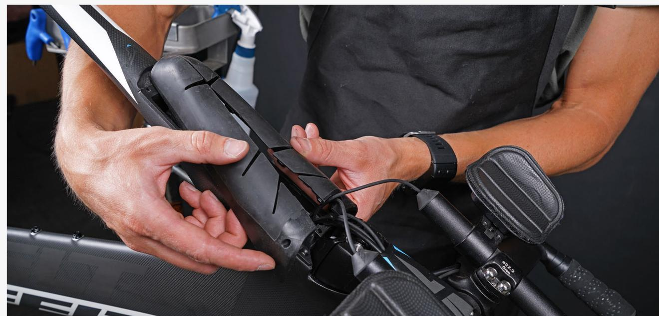
**Step 4:** Flex the two halves of the Calpac top outward to free from cables and remove.
