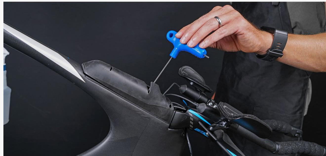
**Step 2:** To simplify the rear brake cable routing, begin by removing the CALpac storage box by unscrewing the (4) internal screws and (1) front screw with a 2.5mm hex wrench.
