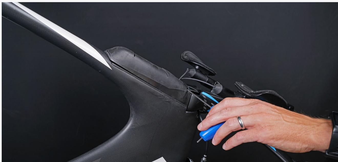
**Step 3:** Unscrew the front side screw on the side of the CALpac to separate the two halves of the box cover.
