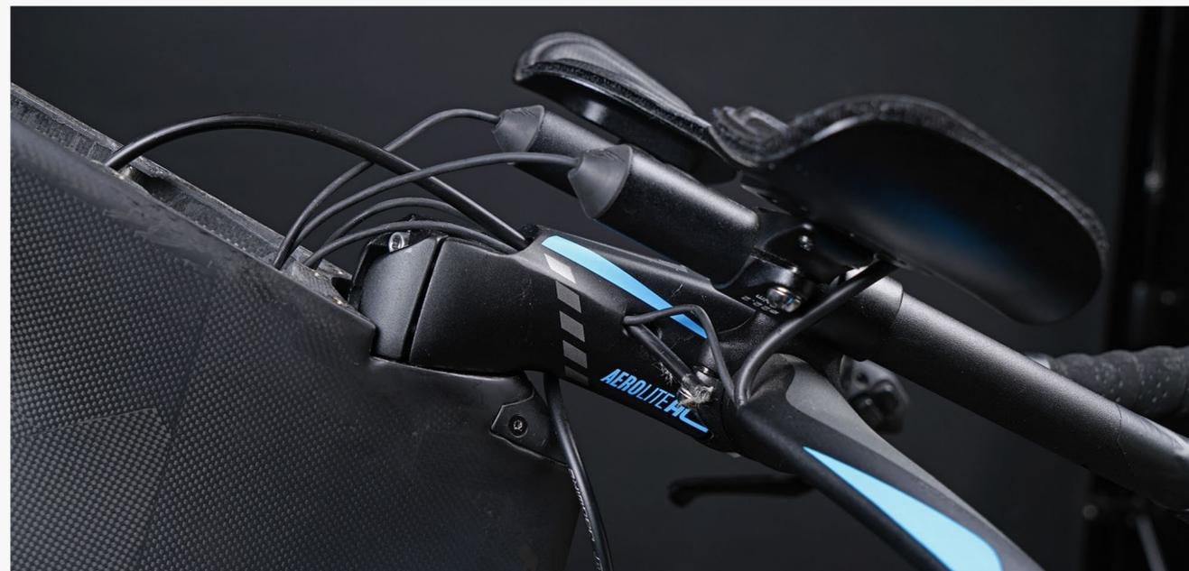
**Step 8:** Guide the housing that you inserted in Step 5 over the inner wire.
