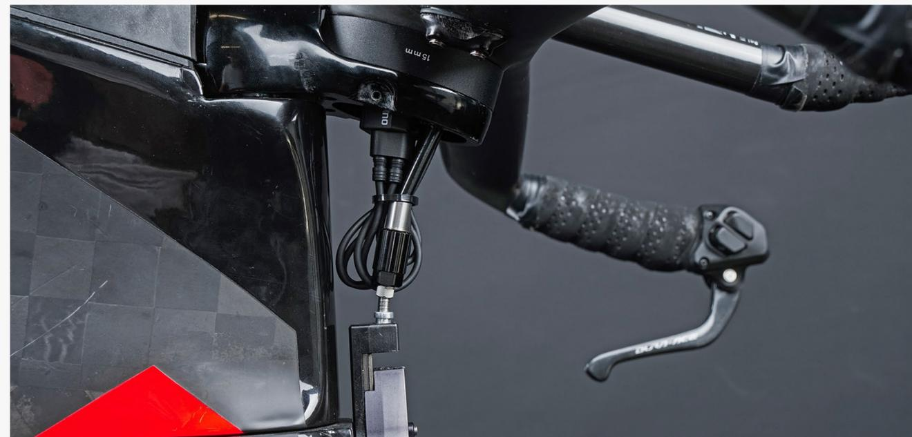
**Step 2:** The A junction is located under the upper brake cover.
