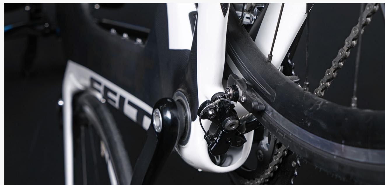
**Step 12:** Install the new inner wire in the caliper per your caliper manufacturer's instructions.
