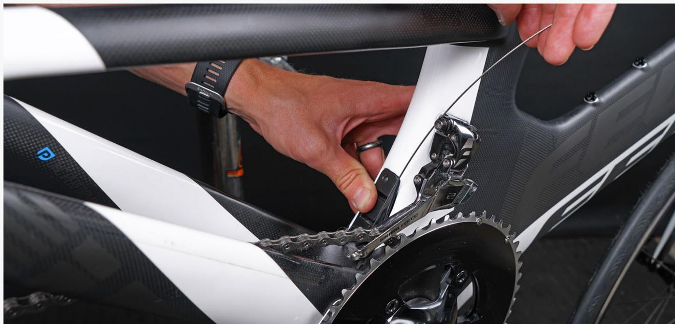
**Step 5:** Carefully reinstall the BatPac while pulling up on the inner wire. Make sure that the housing end remains inside the cable stop.
