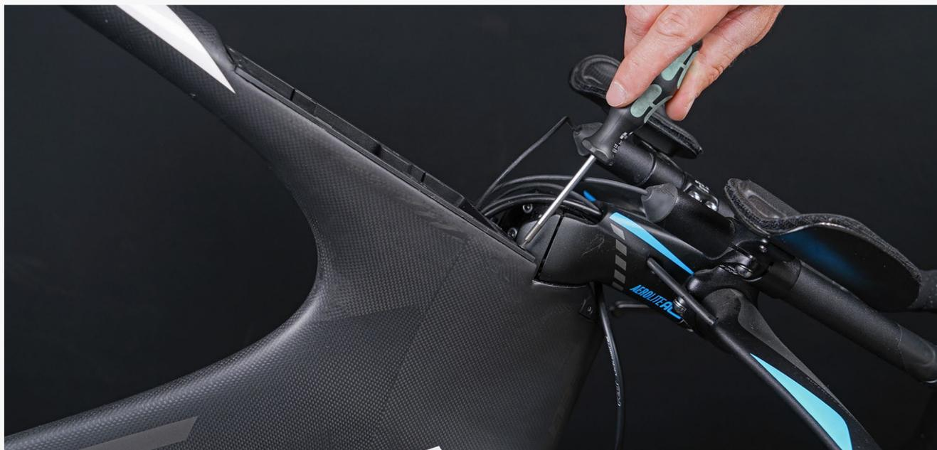
**Step 5:** Using a T9 torx wrench, remove the (2) screws that hold the lower box in the frame and pull out the box. If you have an older model bicycle, you may need to use a 2mm hex wrench instead.
