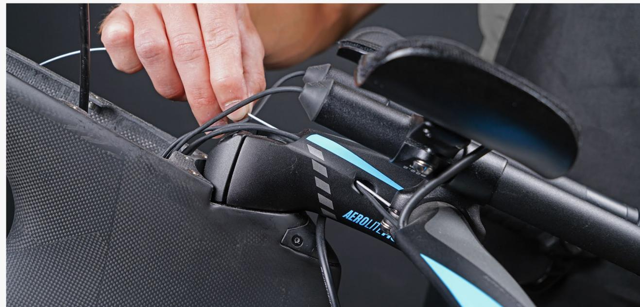
**Step 7:** To route the new housing through stem begin by inserting a spare inner wire from the back of the stem and through the side port entry hole.
