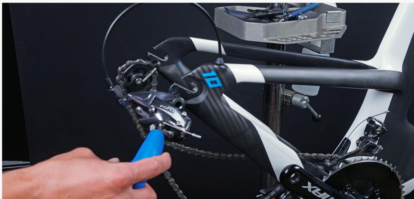
**Step 1:** Loosen the rear derailleur cable screw and remove the inner wire.
