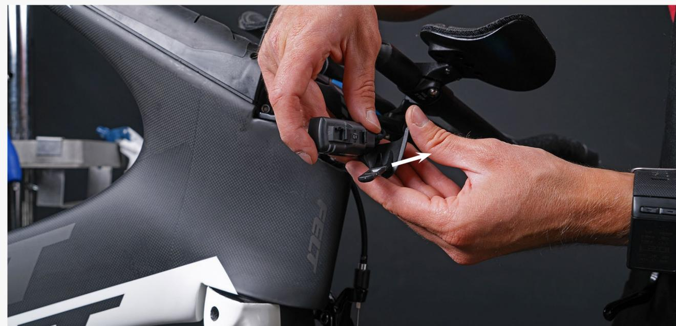
**Step 4:** Slide the A junction sideways to detach from the nose cone.
