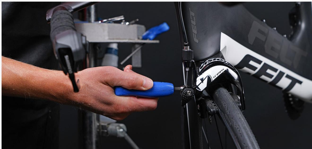
**Step 1:** Loosen the pinch bolt and remove the brake wire.
