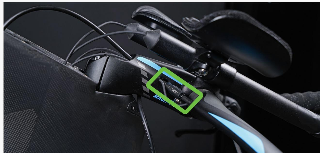
**Step 10:** Install the inline adjuster between the handlebar exit port and stem entry port.
