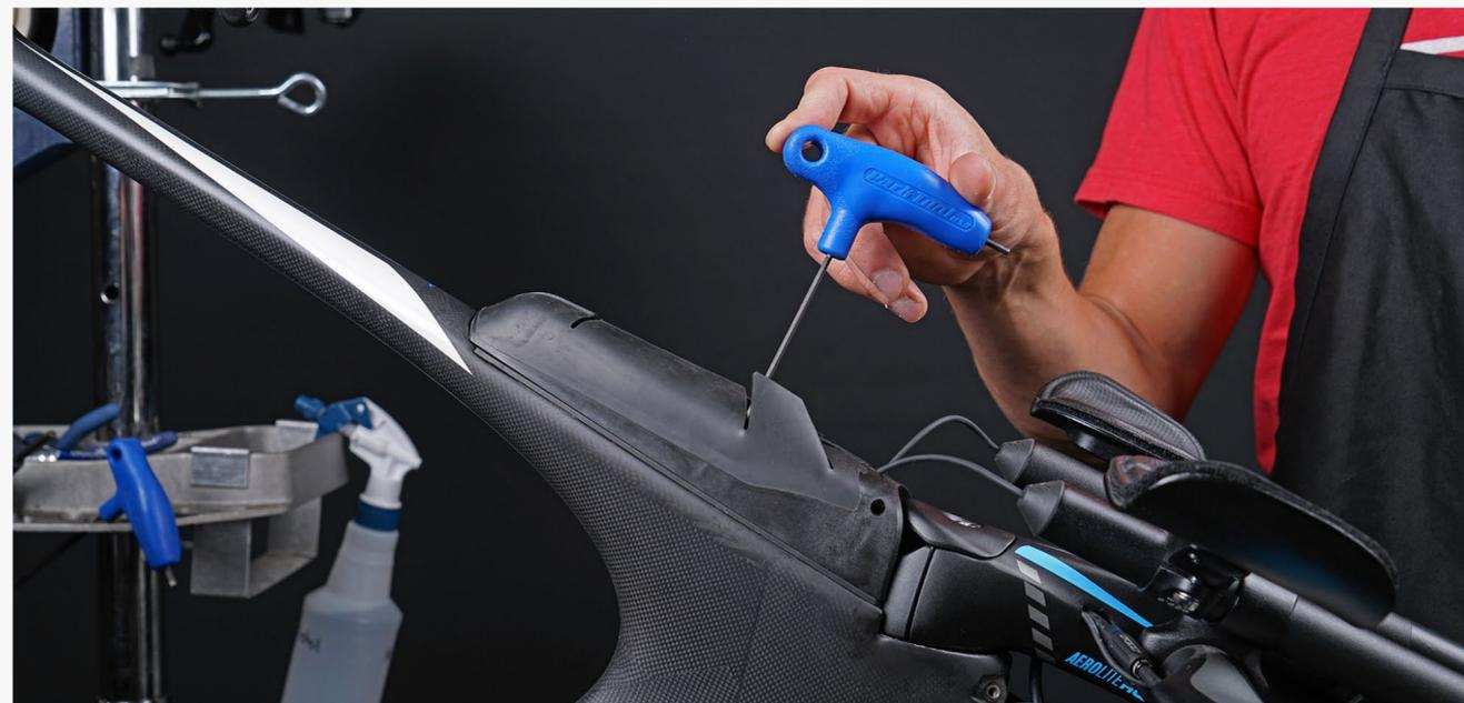
**Step 6:** Remove the CALpac from the frame. Refer to Steps 1-4 in the rear brake cable routing section of this manual.
