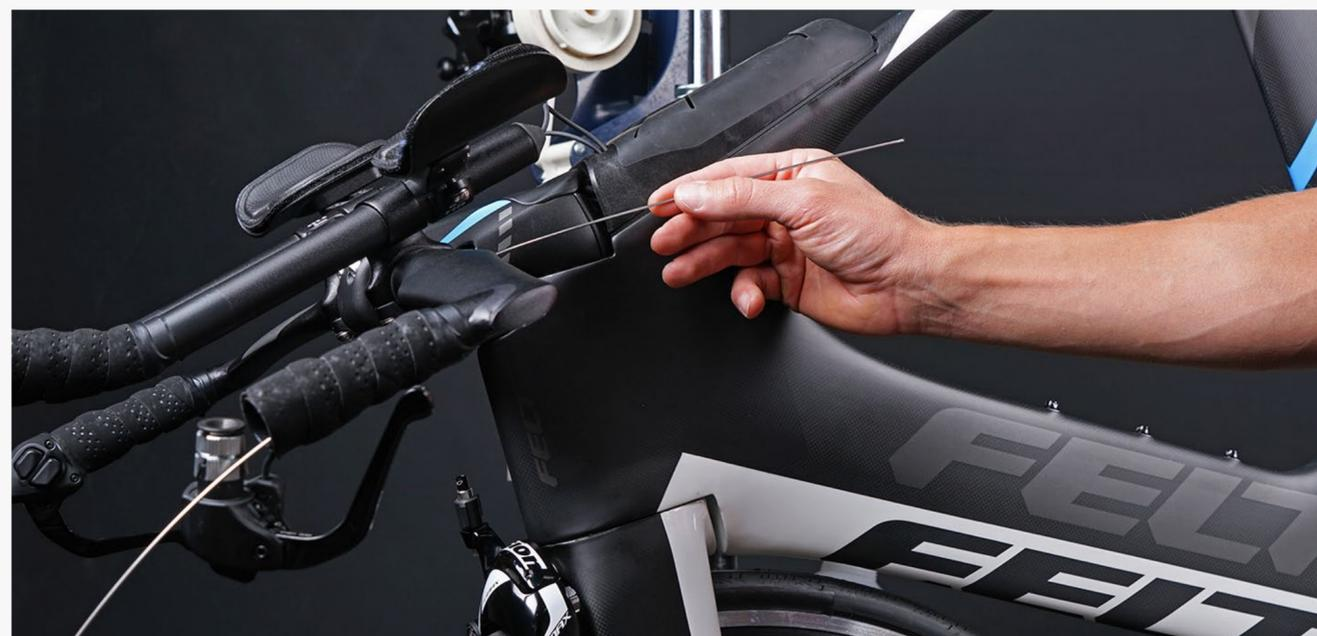
**Step C:** Remove the housing while leaving the inner wire as a guide.
