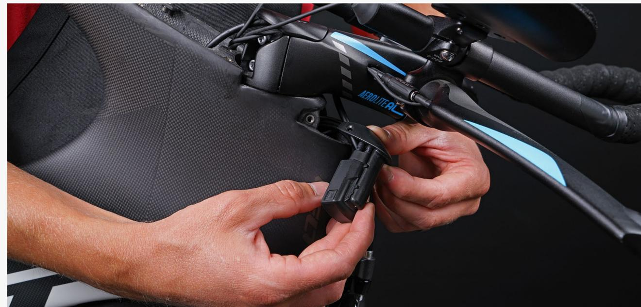
**Step 8:** Connect the wires to the A junction box and slide the junction box onto the nose cone with the wires pointing up.
