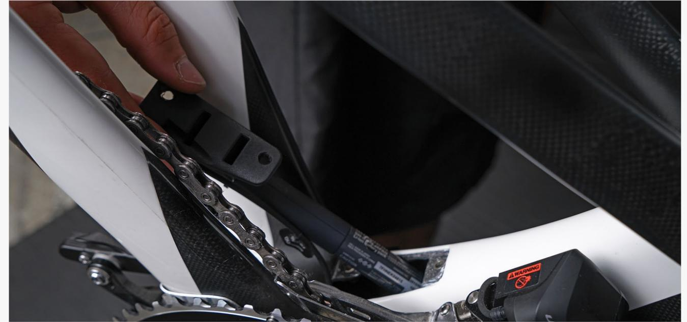
**Step 6:** Insert into the BatPac with attached battery into the frame starting with the top of the battery.
