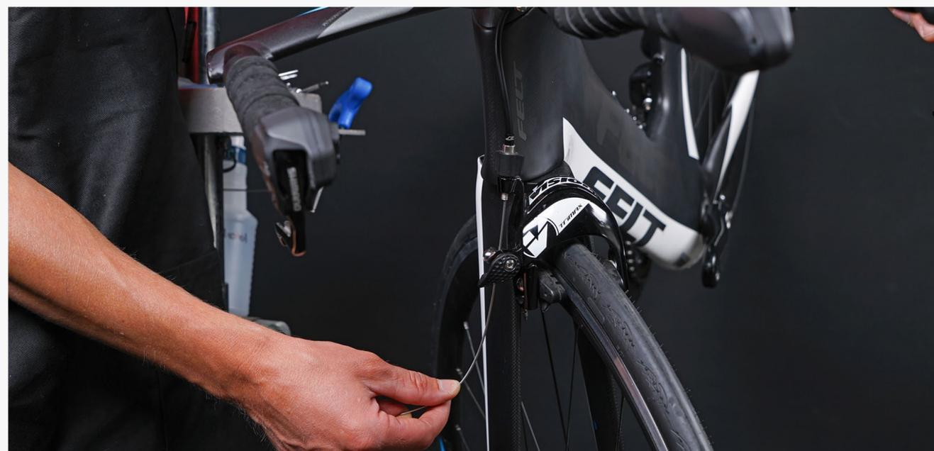
**Step 4:** Secure the inner wire in the brake caliper. Tighten to the specifications recommended by the caliper manufacturer.
