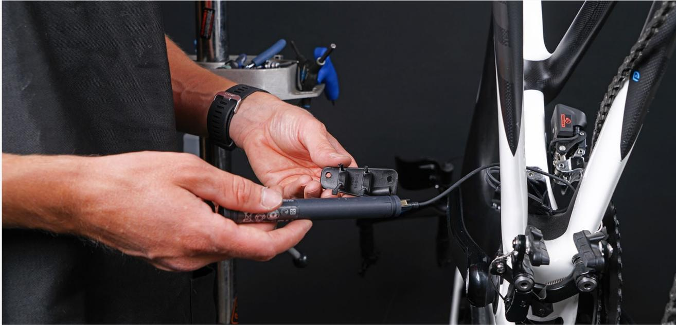
**Step 5:** After performing necessary service, reattach the battery to the BatPac by using (2) small cable ties. Trim excess.
