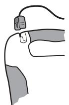
The *DDU-100* AED defibrillation/monitoring pads are supplied sealed in a pouch with the connector and part of the cable exposed. This allows the pads to be stored in a pre-connected state for rapid deployment during an emergency.
