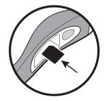
pulling it the rest of the way out. To install a new DDC, insert the DDC, label side up, in the thin slot on the top of the opening for the battery pack. The card should click into place and be flush with the surface of the slot. If the card does not push in all the way, it may have been inserted upside down. In that case, remove the card, flip it over and try inserting it again.
