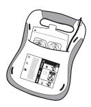
facing up and out, rounded end first, into the pad holder compartment on the back of the AED. When the pad pack is fully inserted, press the pad cable into the groove in the back of the unit to hold it in place and tuck any excess cable behind the pad package.
