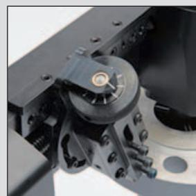
Tool bit fine depth adjustment
