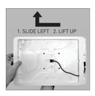
2. While still pinching the clips, flip the Head Unit over and slide the faceplate left, away from the home button, and lift up to remove the faceplate.
