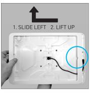
2. While still pinching the clips, flip the head unit over and slide the faceplate away from the home button and lift up to remove the faceplate.
