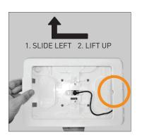
**B.** While still pinching the clips, flip the Head Unit over and slide the faceplate left, away from the home button, and lift up to remove the faceplate.
