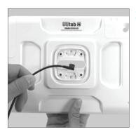
2. Thread the charge cable from the top of the mount pole through the opening located in the center of the Head Unit and pull through to the front side.
