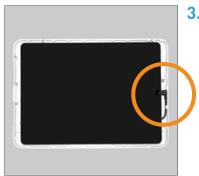
**3. Insert your tablet.** Lay the Head Unit face up and connect the charge cable.
