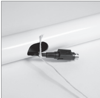
Figure 2. Pull the printer's power cable through the opening located in the middle of the post.
