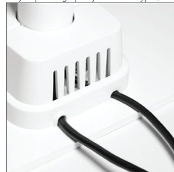
Figure 3. Charge cable and printer power cable exiting the rear of the Base Housing.
