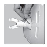
Neck Security Cover. After you attach the Head Unit, slide the security cover up and secure in place using the two (2) M3x10mm Security Cover Screws and Silver L Key.
