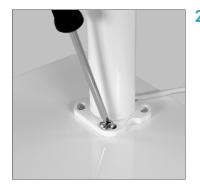
Attach Compact Base. Line up the bottom of the mount pole with the four (4) screw holes in the compact base. Attach using the four (4) Compact Base Screws.
