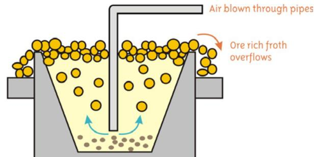
Bubbles form as the air is forced out the bottom of the pipes. These bubbles then rise to the surface of the cells. As the bubbles rose, sulphide minerals would cling to the bubbles and rise to the surface. This was due to the chemicals which had been added. One chemical (called a 'frothing agent') was added to create a frothy mass of bubbles. The other chemical (called a 'collector') essentially waterproofed the valuable minerals and made them stick to the bubbles.
