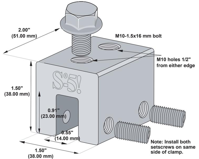
Bolt and washer (or flange bolt) and setscrews included with part
