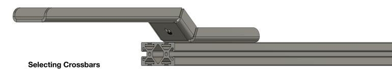
For the most stability of your rod locker you want the brackets as far apart as possible. It's also important for jointed (two piece) rod lockers that you have a bracket on each side of the joint. This will keep the stress at a minimum on your rod locker.
