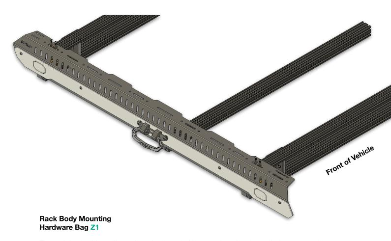
The rack body sides will attach to the threaded inserts placed at the end of your cross bars.
