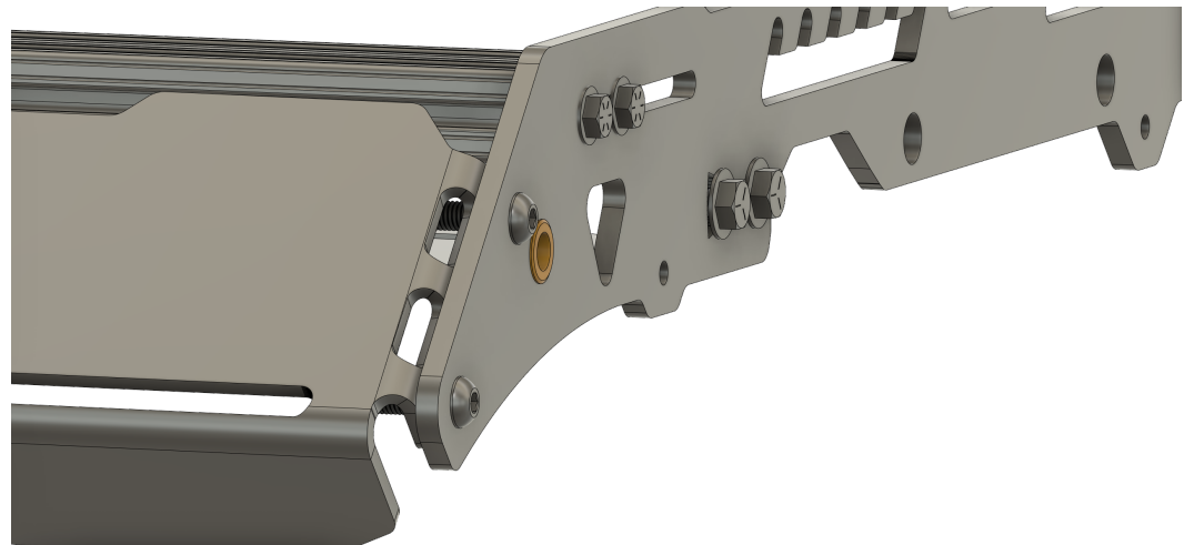
Figure 17 Fairing Installation 1069 Driver Side Shown
